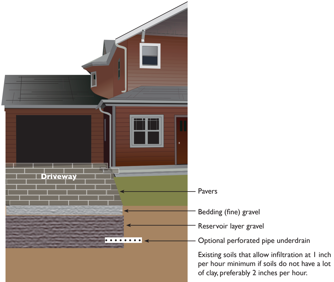
Figure 3.1. Overview of a typical Permeable Hardscape
